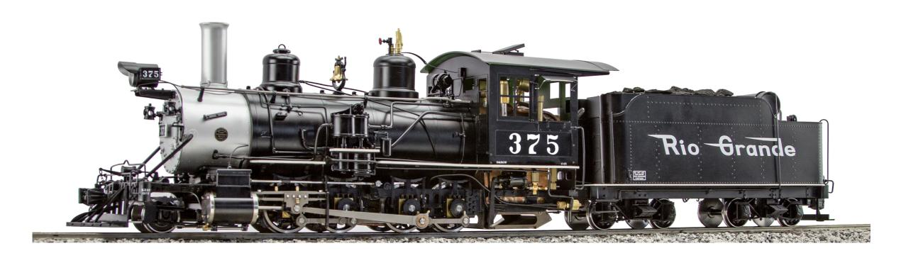
D&RGW C-25, a 2-8-0 or Consolidation type, originally existed as # 103 of the Crystal River Railroad, a narrow gauge line located in the Elk Mountains of central Colorado. It was built in 1903 as C/N 21757 of the Baldwin Locomotive Works, had 33" drivers, 18x20" cylinders, and a tractive effort just short of 25,000 pounds. It was a standard Baldwin design, and other narrow gauge locos of this size and type were built for railroads in the Western Hemisphere.
